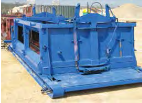
ONSITE BLOCK MOULDS
